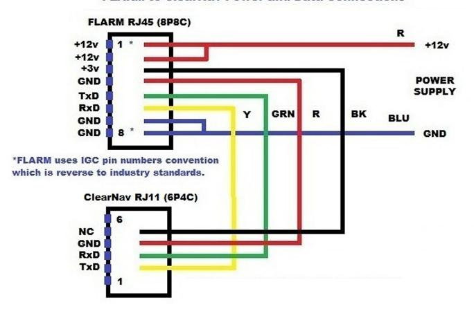
PowerFLARM to ClearNav Data (Power) Cable (Brick) (when Butterfly Display is connected to RJ45 Port)
